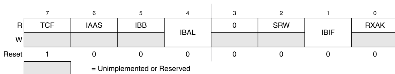
Figure 10-7. IIC Bus Status Register (IBSR)
